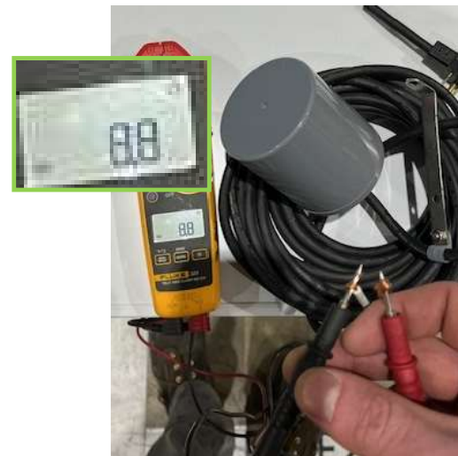
Float in ON Position (8.8 ohms)*
